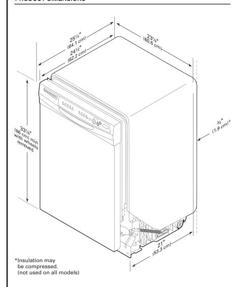
Corner locations require a 2" (5.1 cm) minimum clearance between the side of the dishwasher door and the wall or cabinet.
